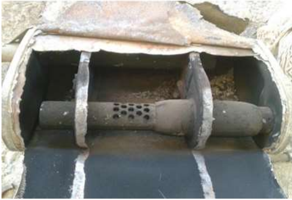
Figure3-2 A detailed examination of the components and operation of a muffler currently on the market.
