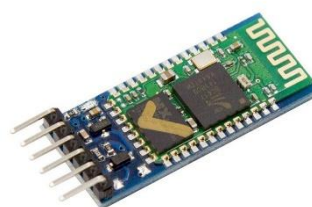
Figure 3. Bluetooth Module (HC05)
