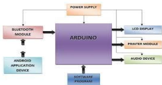
Figure 1. Block Diagram of E-Notice Board
