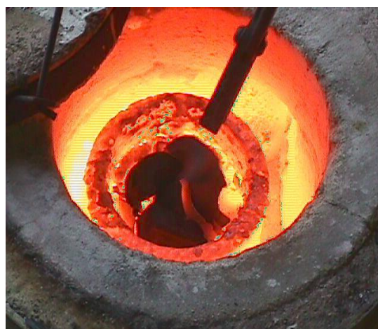
Figure 4: melting the base metal (Al) in the furnace
