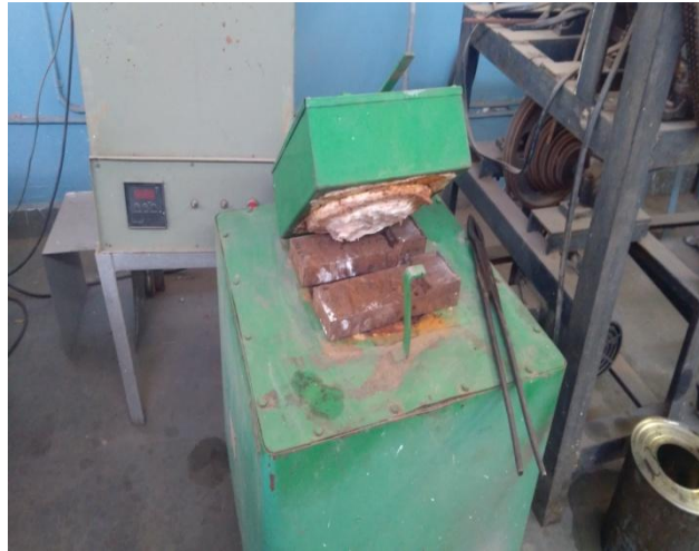
Figure 5: Preheating of mould
