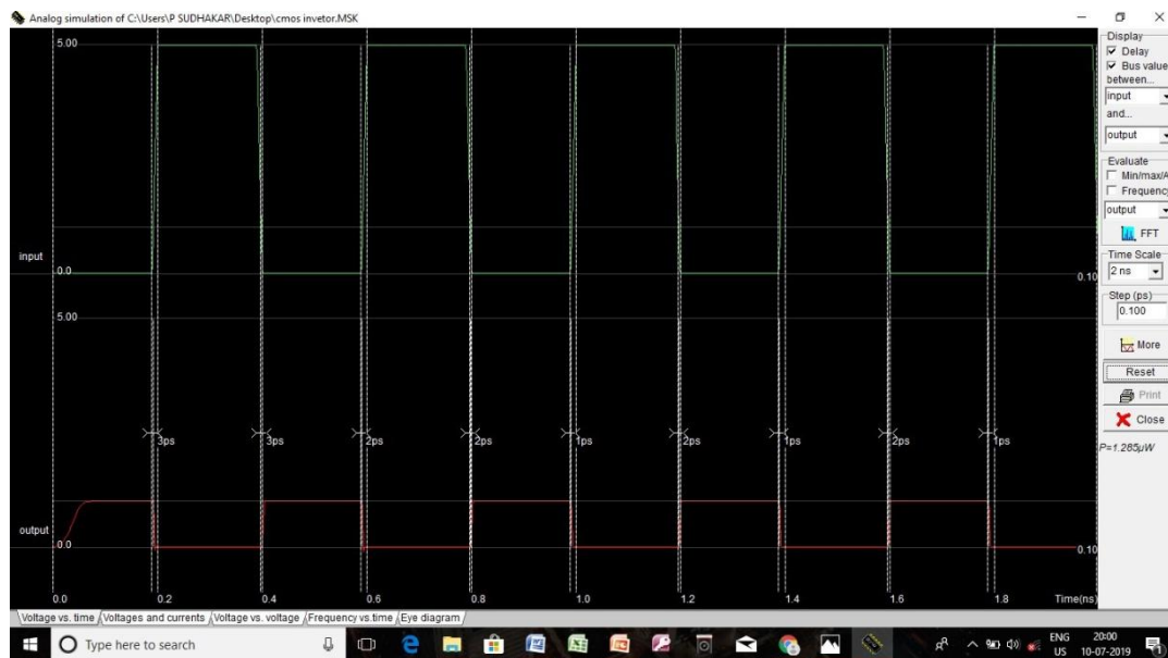
Figure 12: Simulation of CMOS inverter
