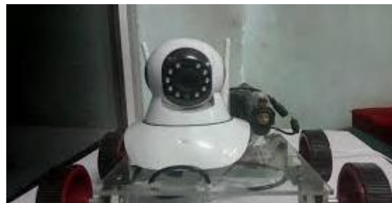
Figure 6. Hardware setup of wireless camera with robot.
