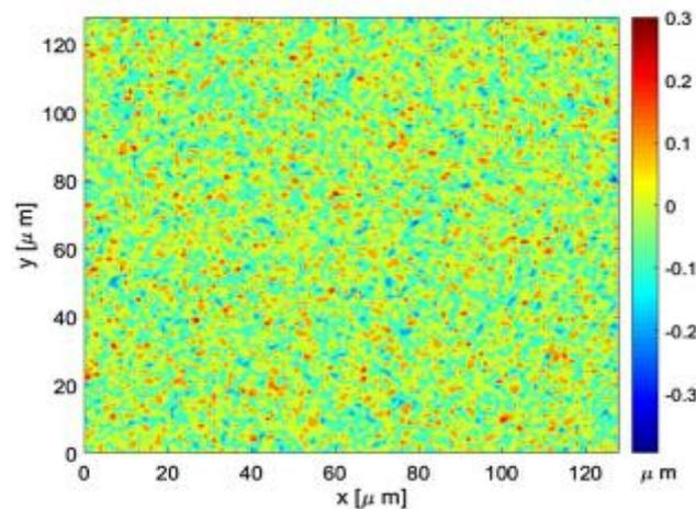
Figure; Topographical contour plot of aluminium surface 2
