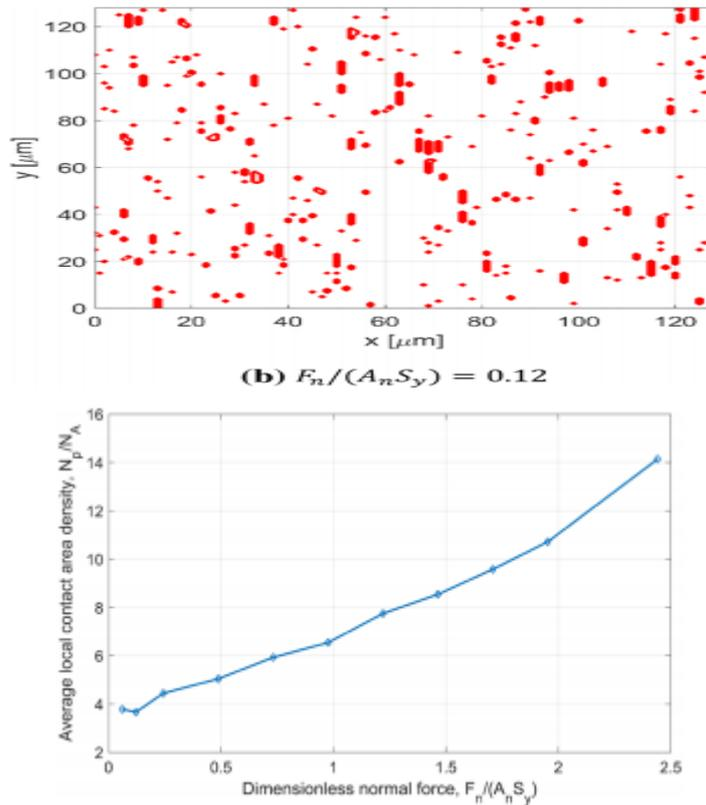
Figure: Average local contact area density versus dimensionless normal force for surface 2
