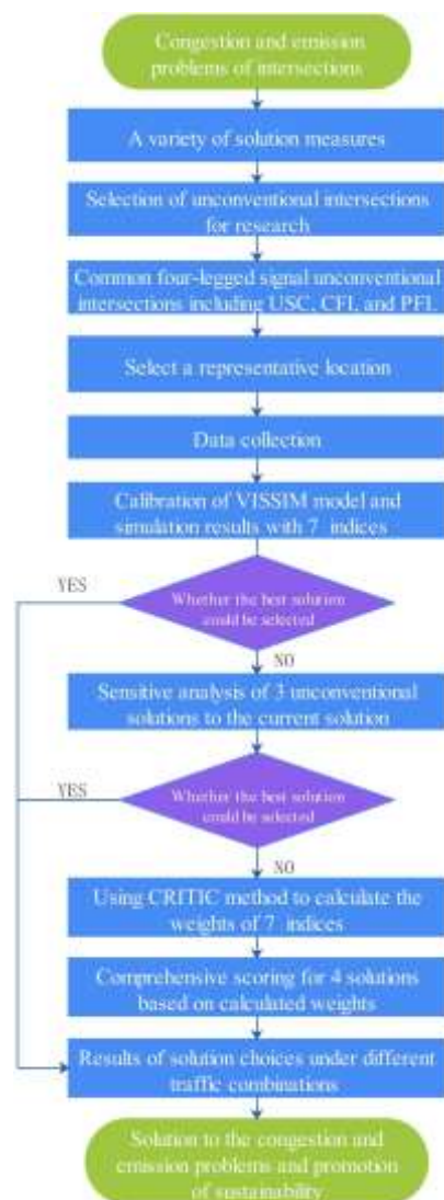
Figure 1. Flowchart of selecting signal unconventional intersections with the CRITIC method.
