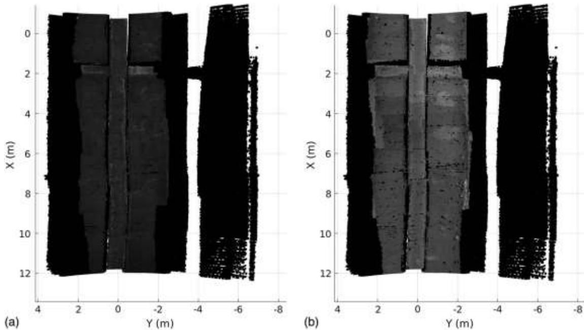
Fig. 15. 3D bridge point cloud with bottom view of deck soffit: (a) cloud colored with vision camera; and (b) cloud colored with IR camera.
