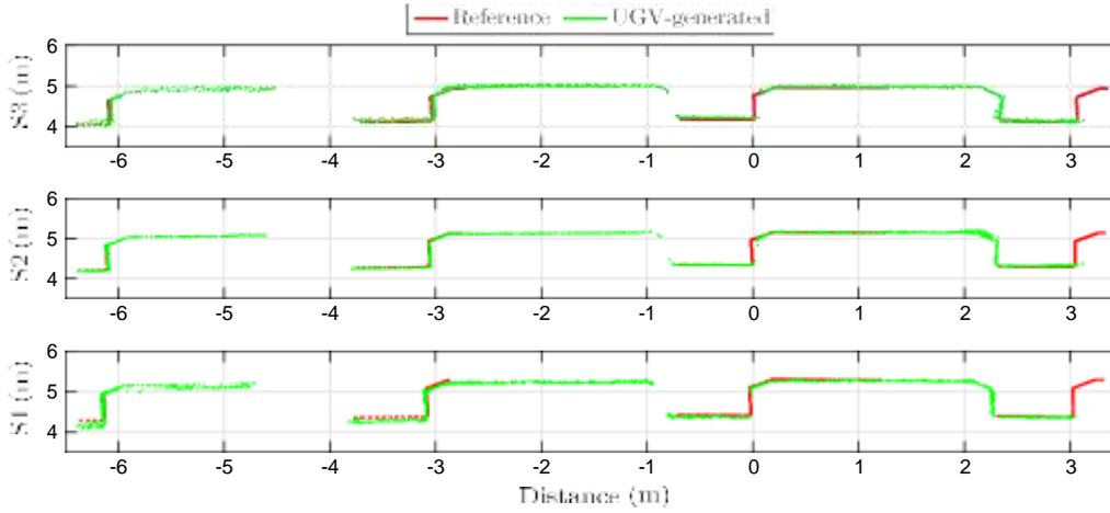
Fig. 12. Cross-section comparison showing the UGV-generated Conestogo River bridge map versus the map generated by the Faro Focus.
