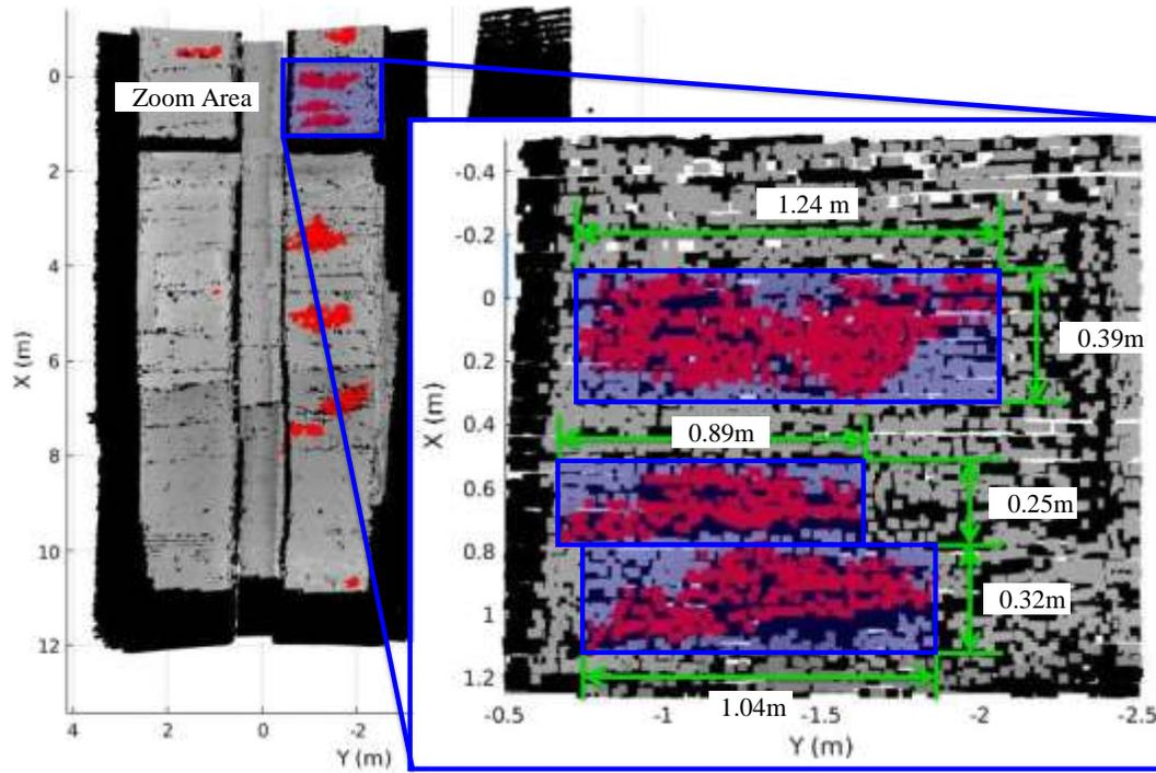
Fig. 19. Point cloud labeled to show delamination sizes.
