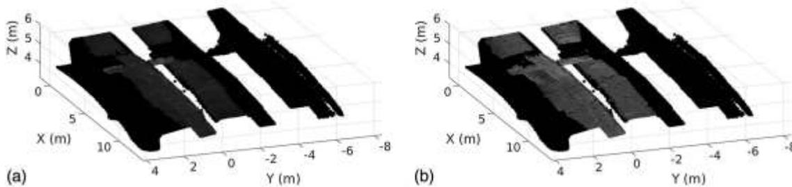
Fig. 16. 3D bridge point cloud with isometric views: (a) cloud colored with vision camera; and (b) cloud colored with IR camera.
