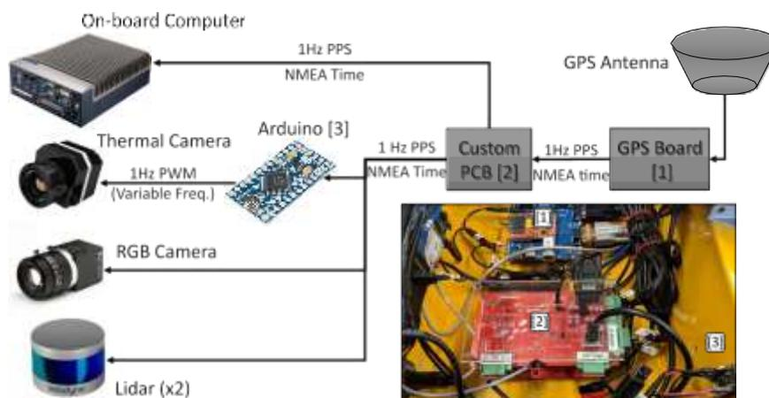
Fig. 2. Sensor synchronization diagram.
