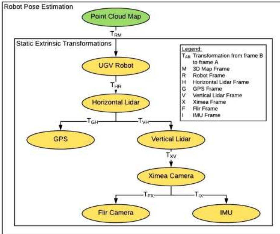
Fig. 3. Robot platform and sensors transformation tree.
