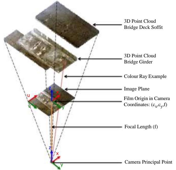
Fig. 13. Point cloud colorization illustration.
