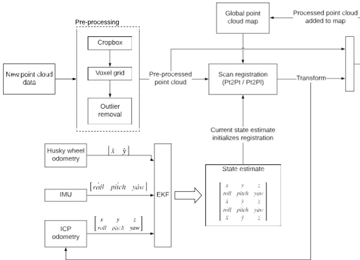
Fig. 6. Conceptual overview of SLAM algorithm.
