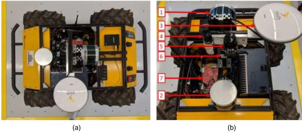
Fig. 1. Details of the sensors mounted on the UGV: (a) Plan view of the sensors and the computer mounted on the UGV along with the custom mount; and (b) labeled sensors: (1) vertical lidar, (2) horizontal lidar, (3) GPS antenna, (4) vision camera, (5) IR camera, (6) IMU, and (7) trigger board.
