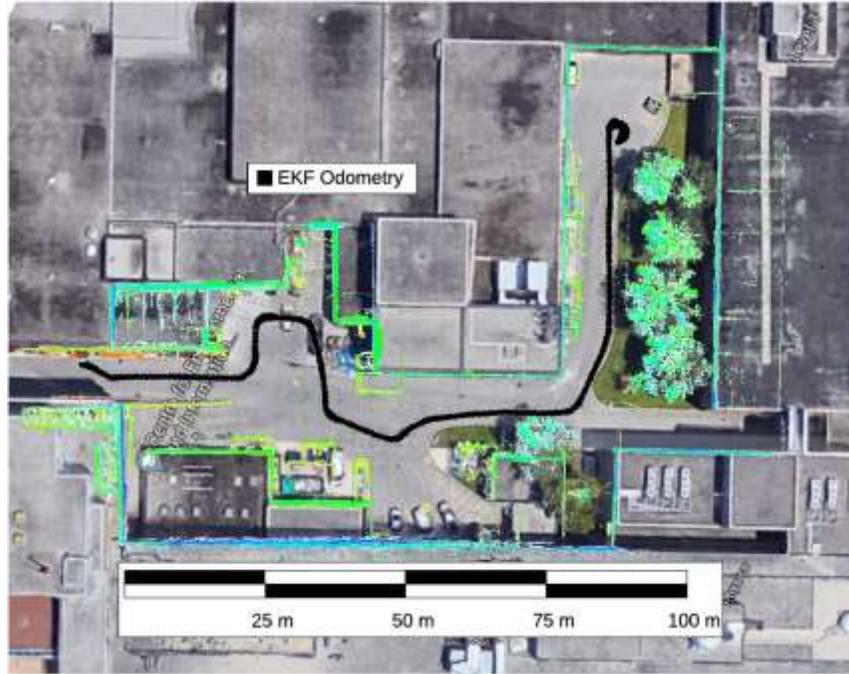
Fig. 7. Satellite view of first test location with overlay of map created using the described SLAM algorithm. (Imagery ©2018 Google, Map data ©2018 Google.)
