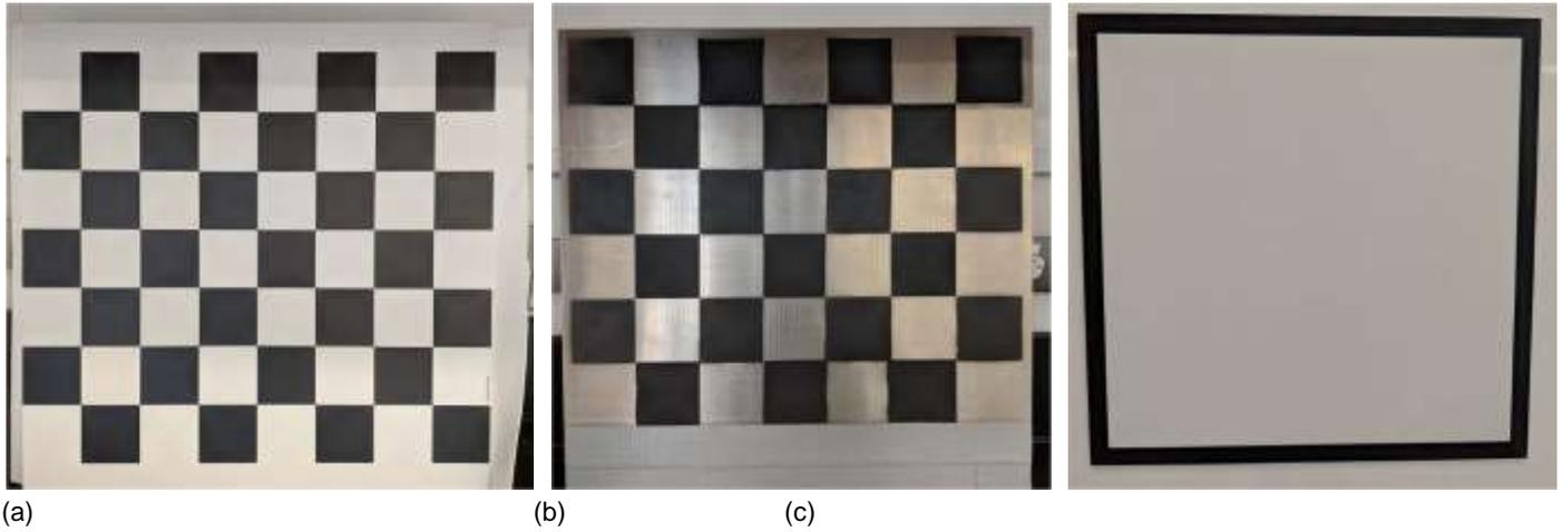
Fig. 4. Calibration targets: (a) vision camera target; (b) IR camera target; and (c) Lidar target.
