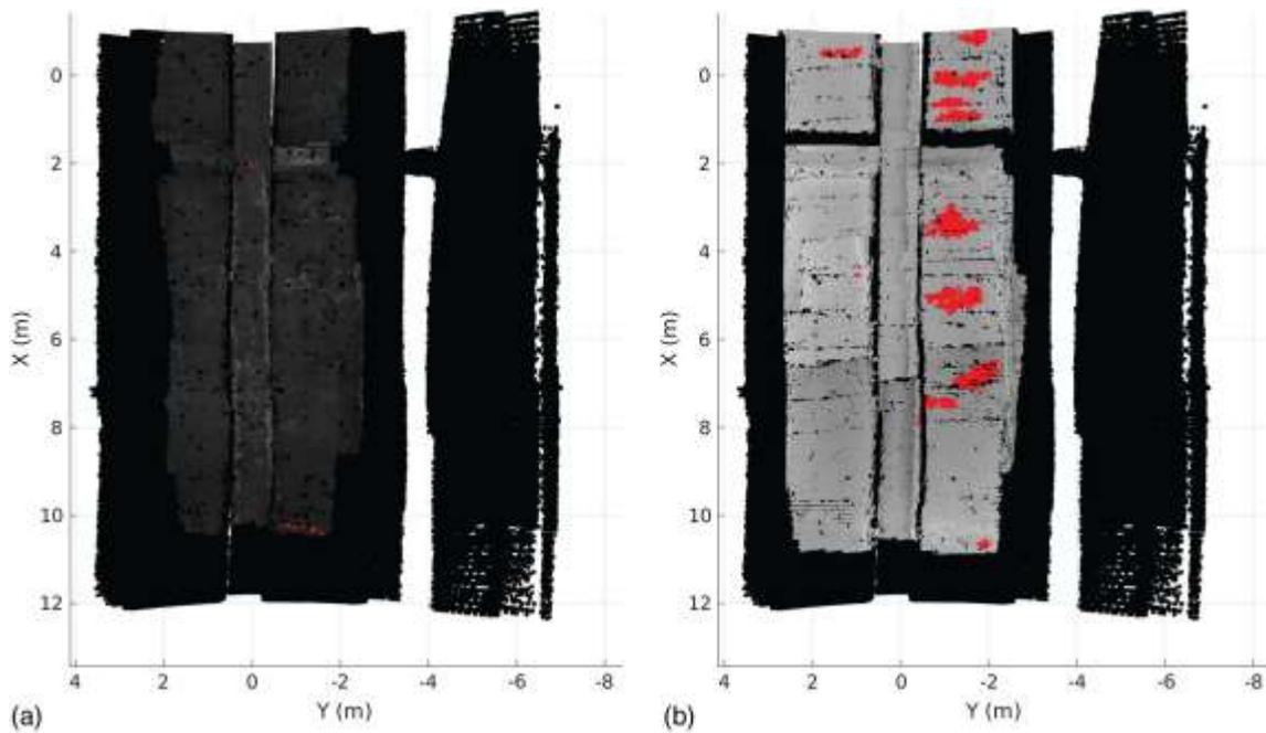
Fig. 18. 3D bridge point cloud labeled with defects: (a) points colored red to show exposed rebar; and (b) points colored red to show delaminations.
