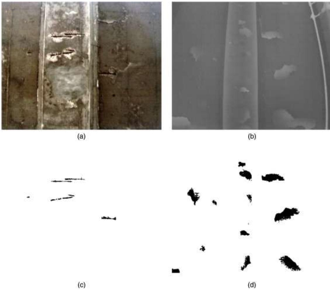
Fig. 17. Semiautomated defect detection using thresholding: (a) vision camera image; (b) IR camera image; (c) detected rebar in the vision camera image; and (d) detected delaminations in the IR image.
