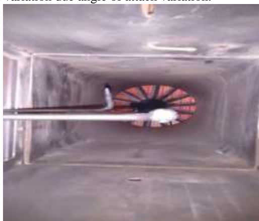
Fig 6.2 Five holes pitot tube
