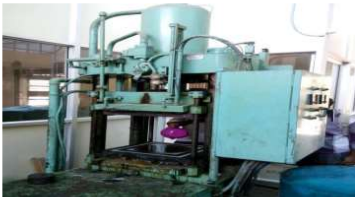
Figure 3 Compression moulding machine used for bio composite.
