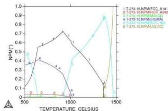
**Figure 2.** Equilibrium diagram of DSS 2507 calculated by Thermo-Calc software. 1.austenite, 2.chromium nitride, 3.M<sub>23</sub>C<sub>6</sub>, 4.sigma, 5.ferrite, 6.liquid.
