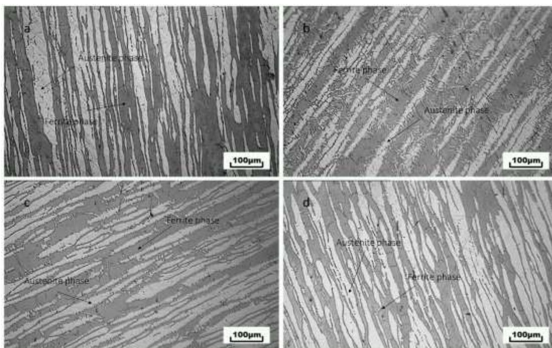
**Figure 3.** Microstructure of DSS 2507 base metal and HAZ specimens after different thermal cycle. Electrolyte: 30% KOH; applied potential: 3V; etching time: 15s. a. base metal; b. single-pass HAZ; c. double-pass HAZ; d. triple-pass HAZ.
