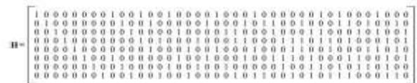
Fig. 8. Parity check matrix for the (40, 32) 3-bit burst with QAEC optimized to reduce the total number of ones.
