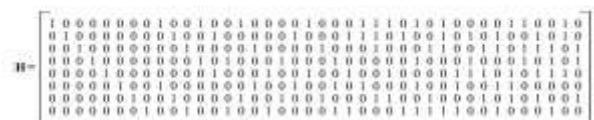
Fig. 9. Parity check matrix for the (40, 32) 3-bit burst with QAEC optimized to reduce the maximum number of ones in a row.
