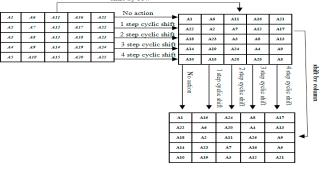
Fig. 3 Circular shift by row and column
