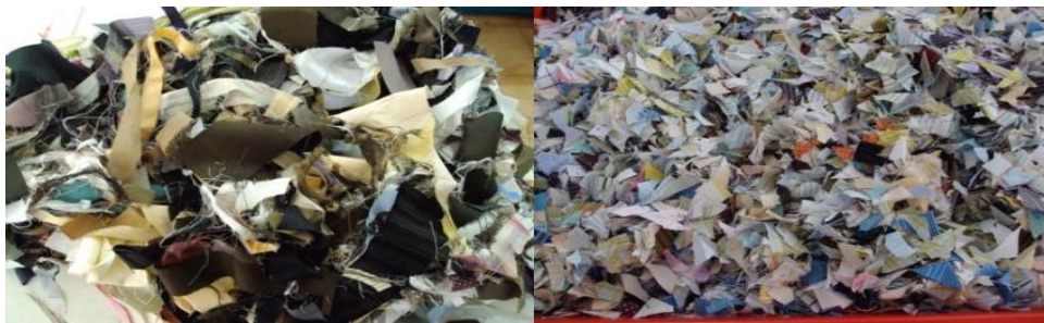
Fig 1: Waste cloth used in concrete
