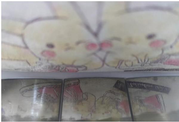
Fig. 7. Finished curved workpieces: position control(top) and hybrid position/force control (bottom)
