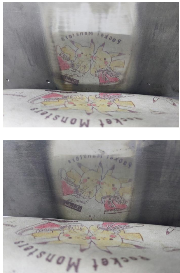
Fig. 6. Finished flat workpieces: position control (top) and hybrid position/force control (bottom)
