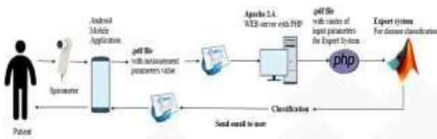
Fig. 3 The architecture of Telemetry System [17].
