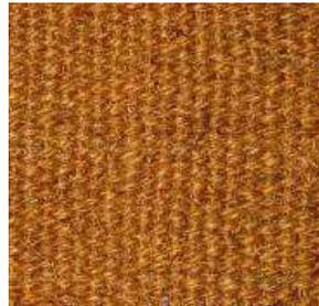
**Figure 3(a):** Coir geotextile Type CWA
