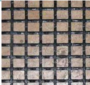
**Figure 2(b):** Biaxial flexible geogrid Type GGF
