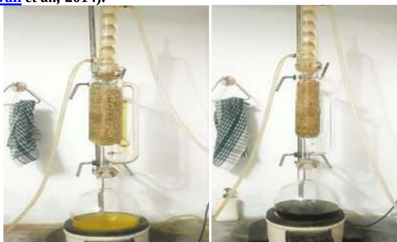
Soxhletation of Helicteres isora (Stem) with Pet. Ether and methanolic solvents
