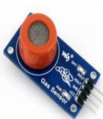
FIG . 2 Alcohol Sensor (MQ-3)
