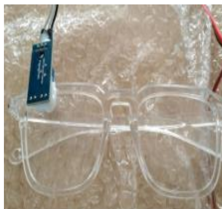
FIG . 4 Eye Blink sensor (IR sensor)
