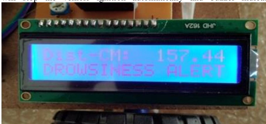
FIG . 11 LCD output drowsiness detection
