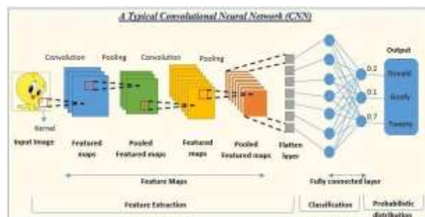
Fig 4 Convolutional Neural Network
