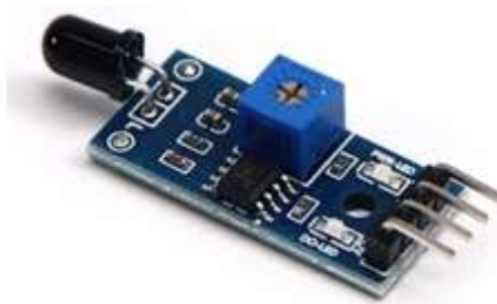
Fig. 3. Infrared flame sensor
