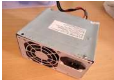
Fig. 6. Switched mode power supply
