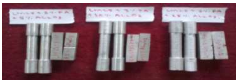
Figure.5: Tensile and impact test specimen with varying composition of Al 2 O 3
