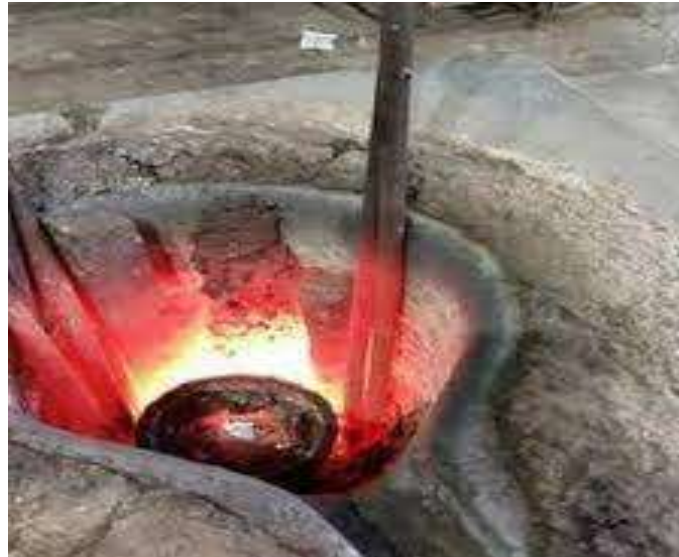
Figure.1: Furnace with Crucible containing LM25.
