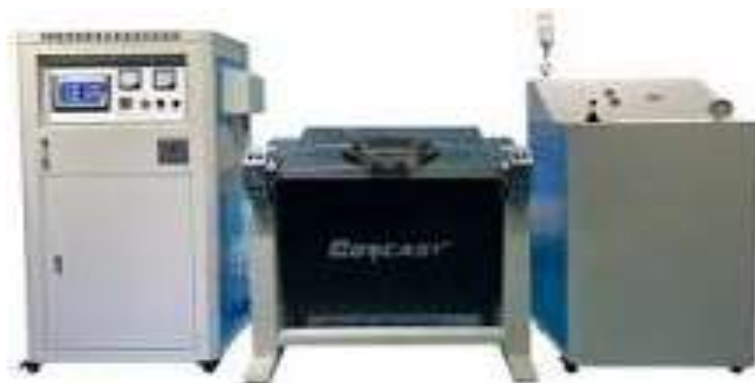
Figure.3: Hydraulic Titling Small Induction Furnace
