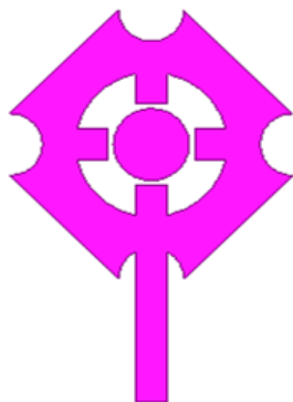
Fig. 11 Inserting a circle slit inside the first circle slot
