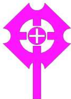
Fig. 13 RPA with a plus-shaped slot inside the second circle slot
