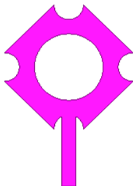
Fig. 7 A circle slot etched in the middle of RPA
