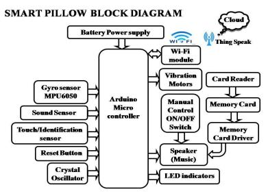
The hardware implementation of the Smart Pillow Project involves the integration of various components to create a functional system. The regulated power supply provides a stable power source to ensure consistent operation. The Arduino microcontroller, connected to a crystal oscillator for precise timing, serves as the central processing unit. It controls and coordinates the functions of different modules. A reset button is included for manual resetting of the system if necessary.
