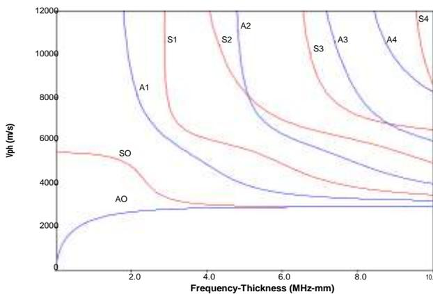
Figure 3: Phase velocity dispersion curve
