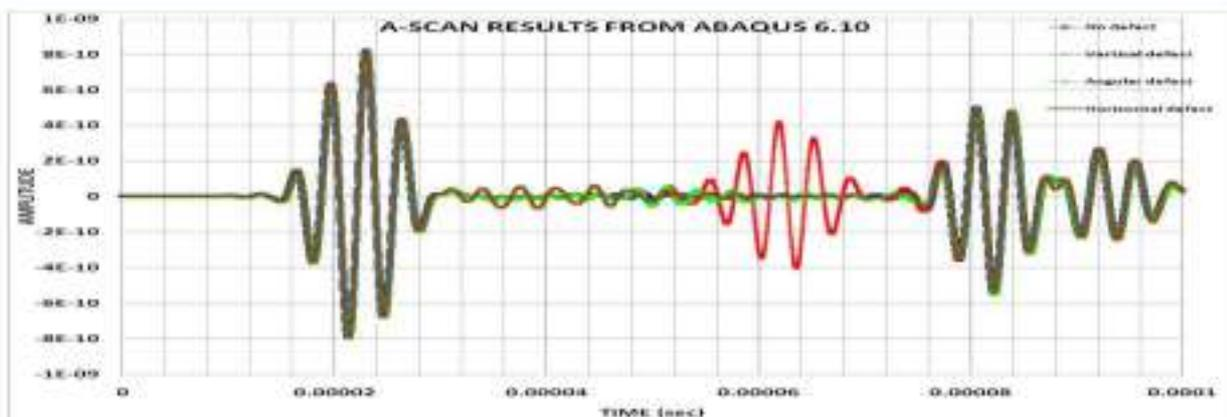
Fig. 9d shows the waveform from a plate with vertical defect. The waveform peak corresponding to the defect occurred around  $0.57 \times 10^{-4}$ s. The amplitude of the peak is quite equal on comparison with the reflected wave peak.
