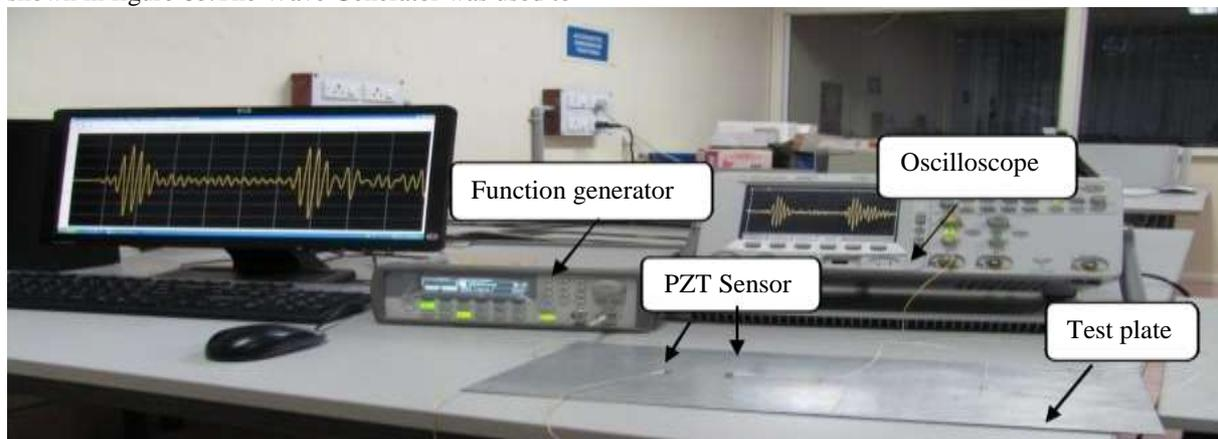
Figure 6: Experimental setup for SHM
