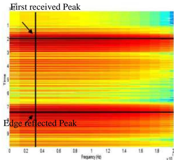
Figure 10: STFT of defect free aluminum plate (time-frequency analysis)
