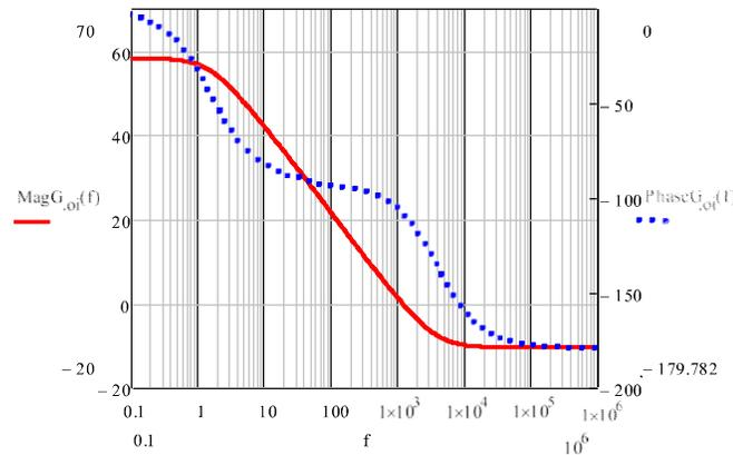
Fig. 7. Bode plot of the open-loop current transfer function.
