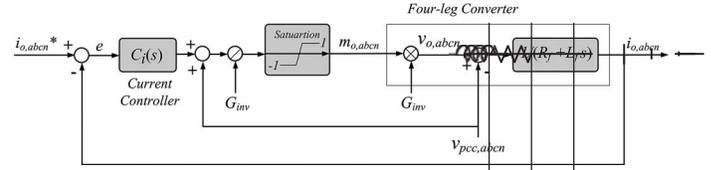
Fig. 5. Block diagram of the current control loop.
