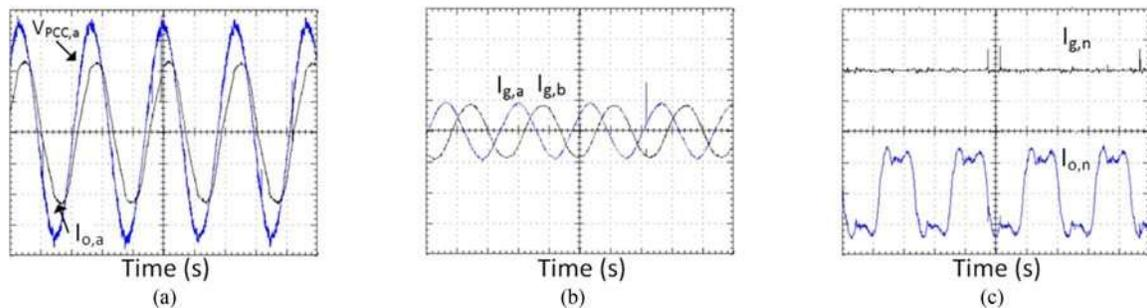
Fig. 14. Active power delivery and nonactive compensation: (a) PCC voltage and inverter currents; (b) two phases of grid current; and (c) grid neutral current ( $I_{g,n}$ ) and inverter neutral current ( $I_{o,n}$ ).
