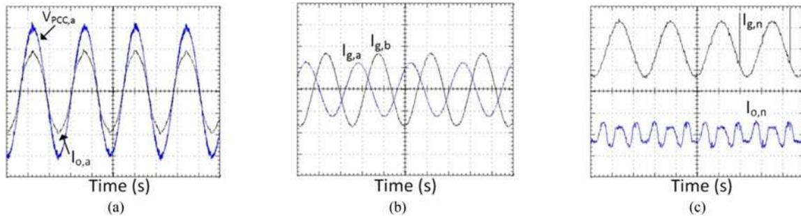
Fig. 13. Active power delivery and void compensation: (a) PCC voltage and inverter currents; (b) two phases of grid current; and (c) grid neutral current ( $I_{g,n}$ ) and inverter neutral current ( $I_{o,n}$ ).
