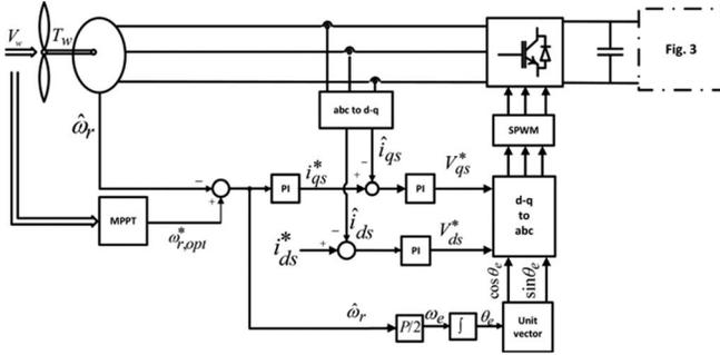
Fig. 2. Control scheme of machine side converter.
