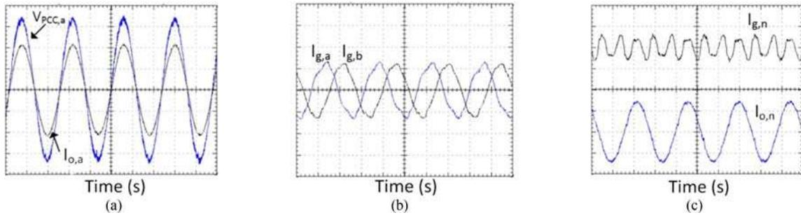
Fig. 12. Active power delivery and unbalance compensation: (a) PCC voltage and inverter currents; (b) two phases of grid current; and (c) grid neutral current ( $I_{g,n}$ ) and inverter neutral current ( $I_{o,n}$ ).
