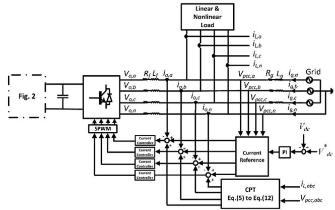
Fig. 3. Control scheme of a grid-side converter.
