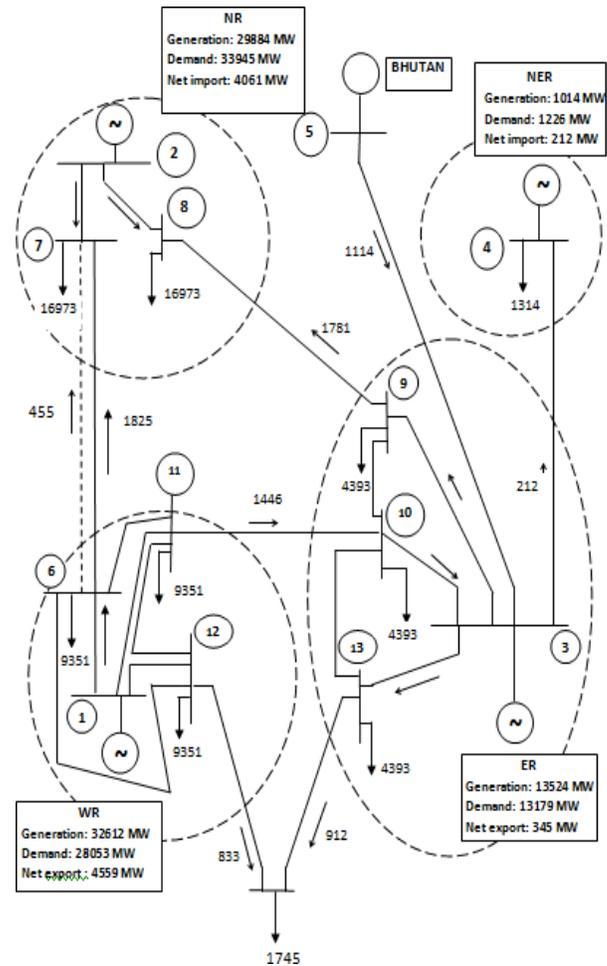
Fig. 5 Tie Line Flows on 31<sup>st</sup> July at 12.30 hrs
