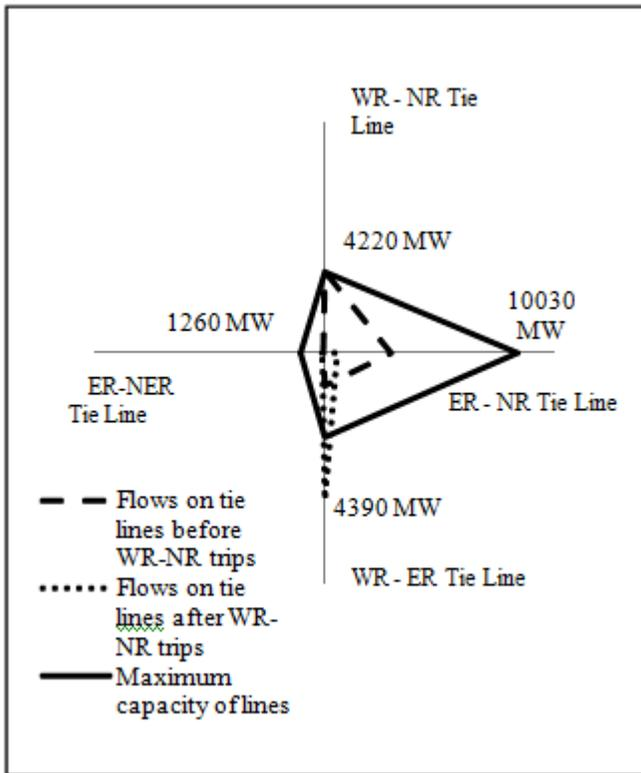
Fig. 8 Tie Line flows before and after WR-NR Tie Line Trips
