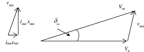
$$v_{mn} = \sqrt{i_{mn}^2 r_{mn}^2 + i_{mn}^2 x_{mn}^2} \quad \delta_{mn} = \frac{v_{mn}}{V} \approx v_{mn} \quad (V \approx 1)$$
