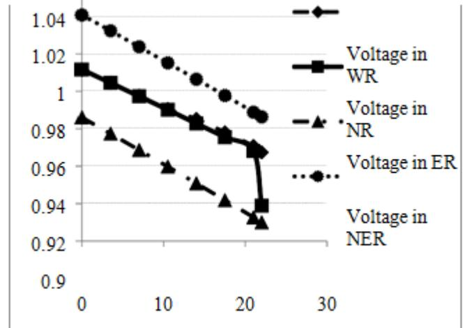
Fig. 7 Average of region-voltages with increase in NR load
