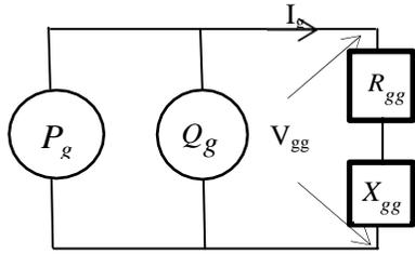
Fig.1. Only one generator feeding the network
