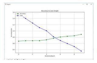
In above graph x-axis represents epoch/iterations and y-axis represents accuracy and loss values. In above graph green line represents accuracy and blue line represents loss and in above graph we can see with each further iteration accuracy get increase and loss get decrease
