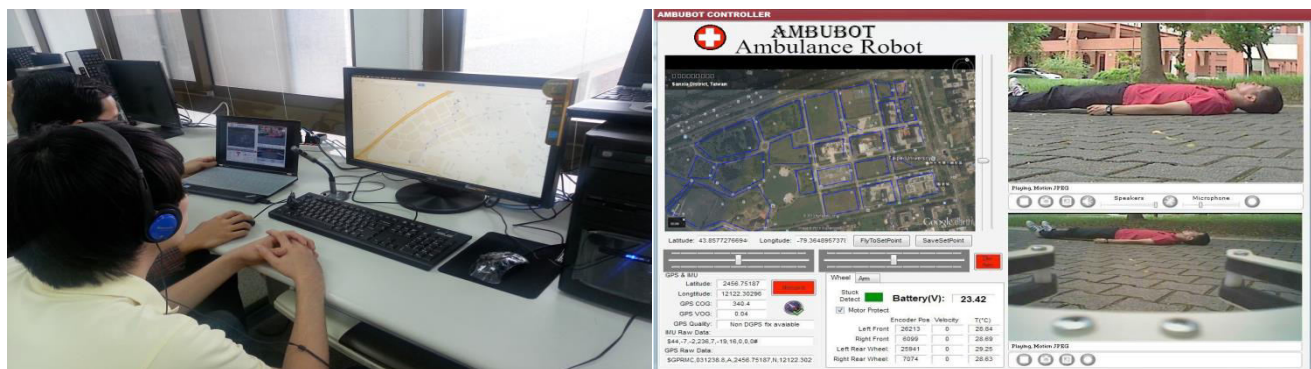
Fig: 4.3 Remote operation of robotic ambulance
