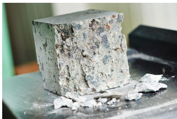
Fig4: Cube Sample broken
