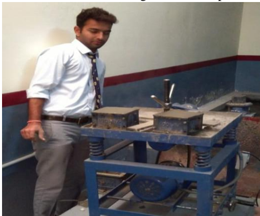
Fig-2 Compaction by Vibrater
