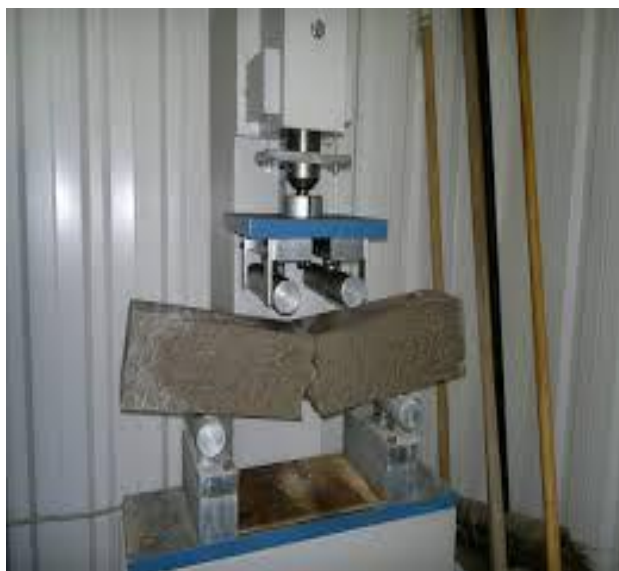
Figure-7 Flexure strength test
